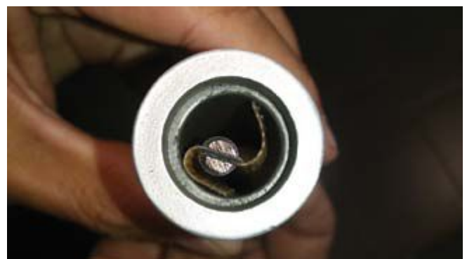
Figure 4. Mid-size roto peen flap (1.25 x 0.56 inch / 31.8 mm x 14.3 mm) in a 0.75 inch (19.1 mm) hole
