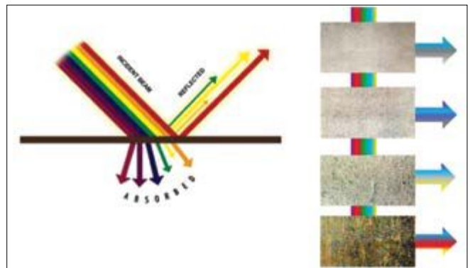
The working principle of WA Clean is color spectrometry. The coordinates obtained are converted to a unique cleanliness level index from 0 to 100.
