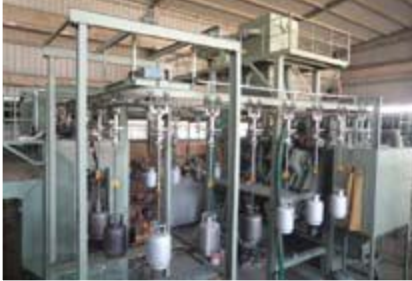
Airless 6 Wheel Machine with Overhead Conveyor
