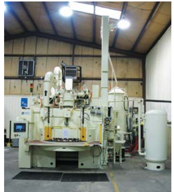
Large 84" Index Unit, 12 Pressure Nozzles
