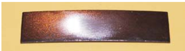
Fig.9. Hand-polished Almen ‘A’ strip showing area of complete indentation removal.
