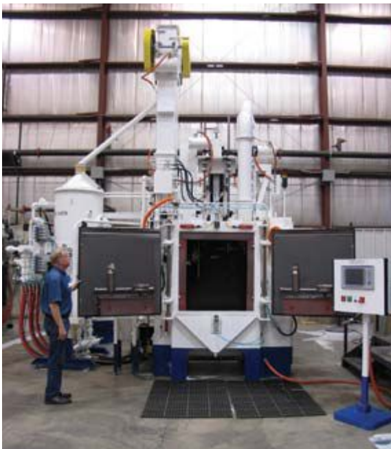
Single Cell Unit, 5 Pressure Nozzles
