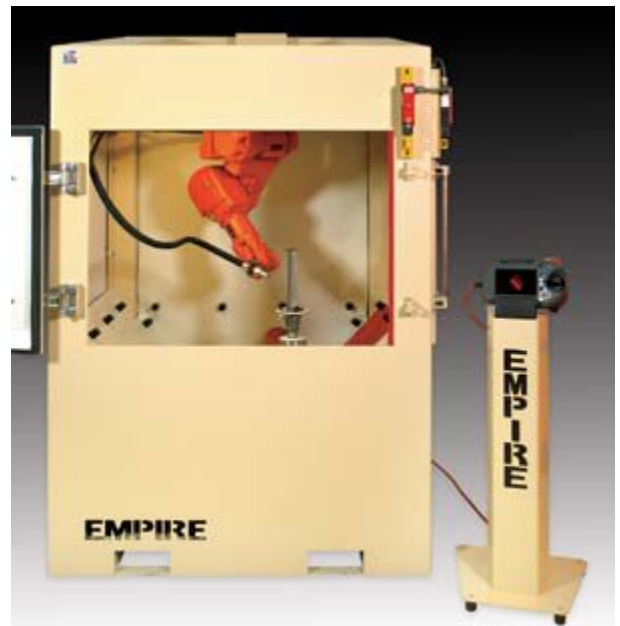
A robotic peening cell with an ABB 6-axis robot to control nozzle movement and a DC or Servo drive to control part movement.
