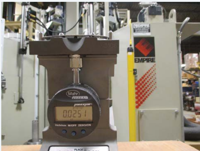
Some blast cleaning operations are using Almen strips to quantify and validate their cleaning operation.
