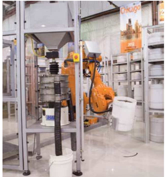
Shotzie "presents" the media for inspection. A SWECO ensures that the media is kept in top condition.
