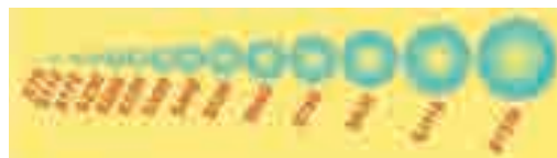
Fig.2 Nominal shot sizes as specified in J444 – with equivalent spheres drawn to scale.
