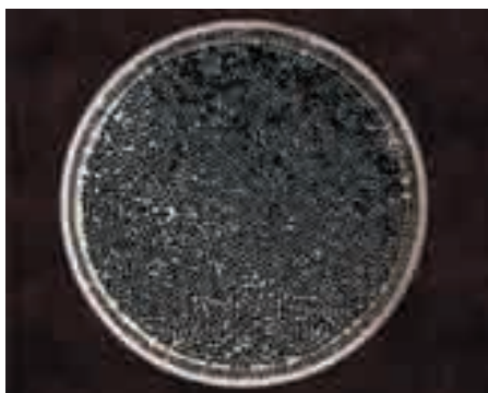
Fig.8 SLR camera image of S330 shot sample viewed through a light box.
