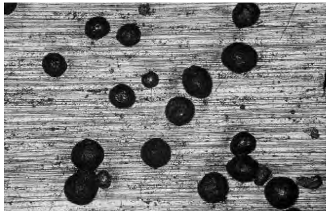
Fig.5 Variability of indent size.
