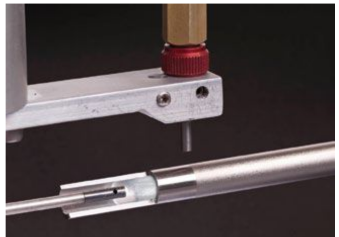
Small ID/OD are peened simultaneously
