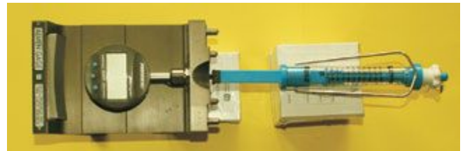
Fig.6. Push/pull spring balance testing resistance force of an EI TSP-3 Almen gage.
