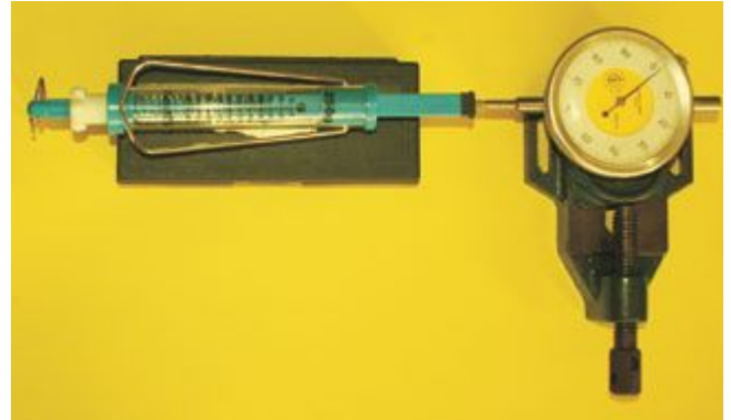
Fig.5. Push/pull spring balance testing resistance force of an analogue dial tip.
