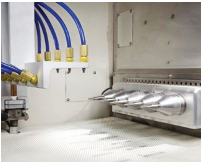
Peening five bone screws simultaneously with small lathe
