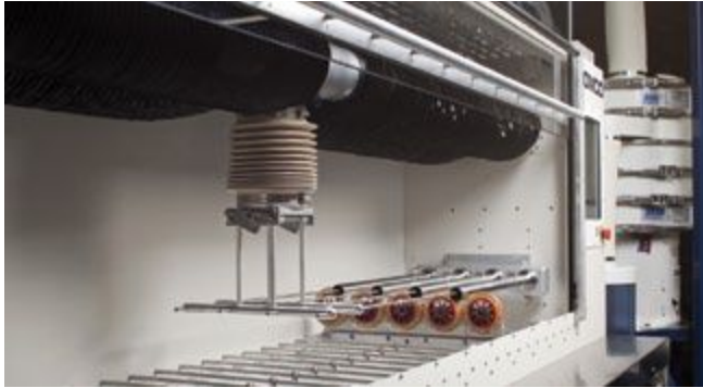
Peening four shafts ID/OD simultaneously for aerospace
