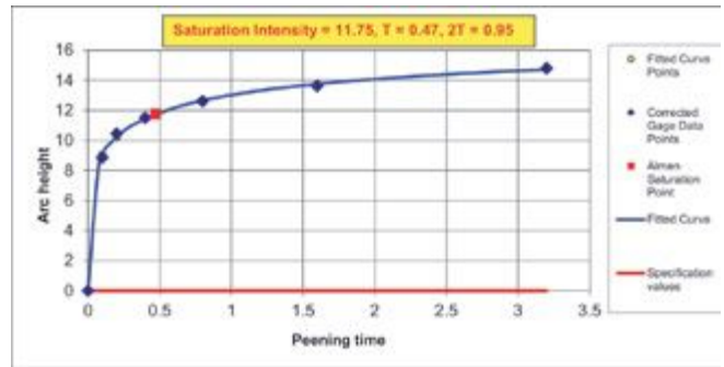
Fig.4. Typical Peening Intensity Curve.
