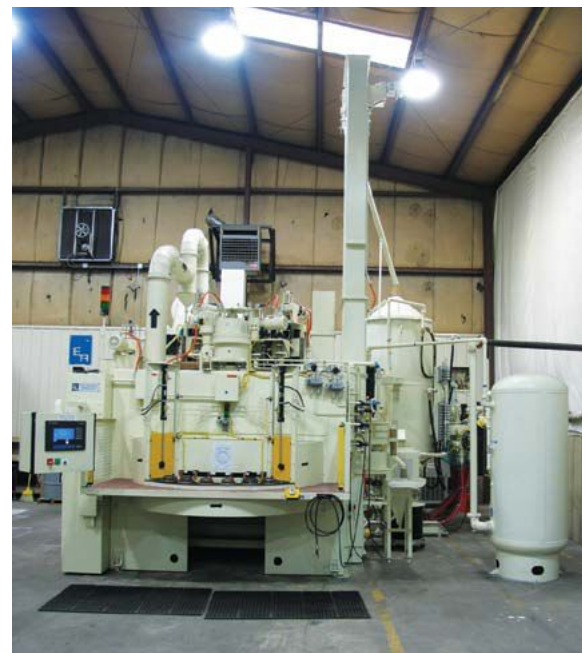
Large 84" Index Unit, 12 Pressure Nozzles
