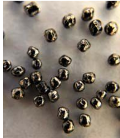
Random sample of conditioned CW shot could include traces of insufficiently conditioned, cylindrical particles.
