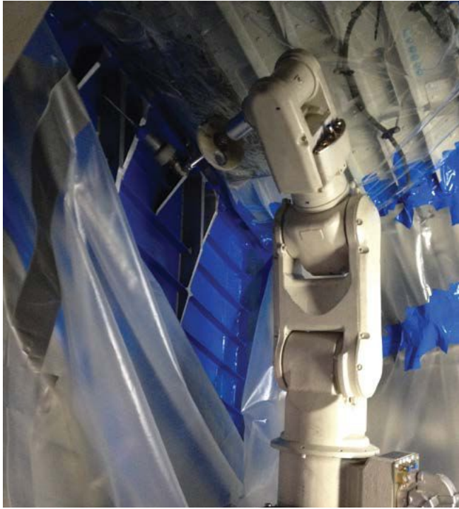
Figure 2: Robotic peening of critical geometry
