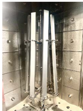
A birdcage-style fixture with multiple long parts fixtured topeen simultaneously
