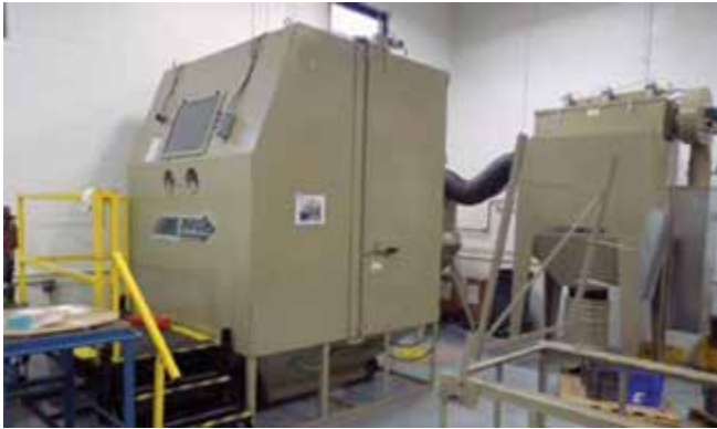
The modified Zero BNP-7212 Suction Blast Cabinet
