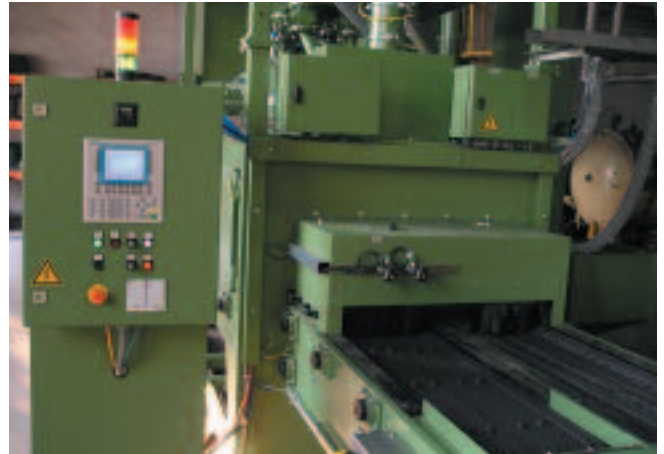
Two parts conveyors ensure the springs are shot blasted on both sides.
