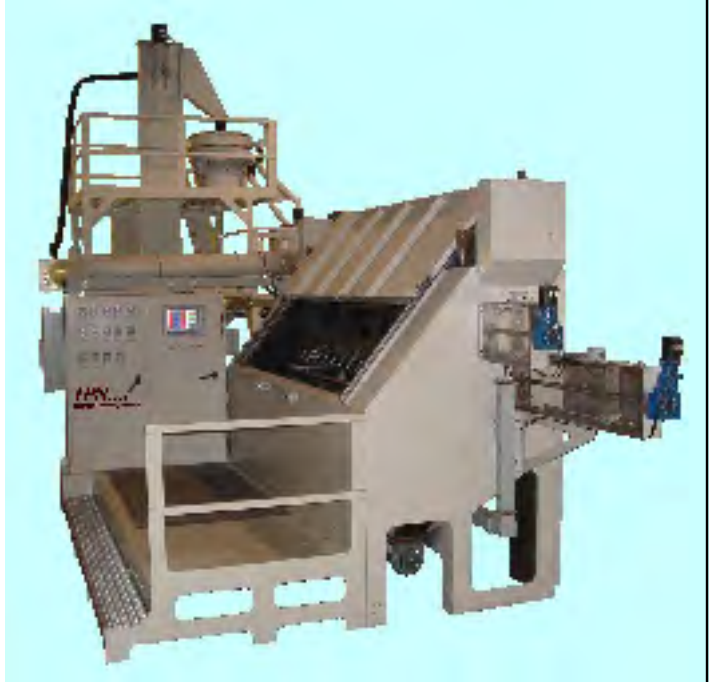
Dual media 14 nozzle shot peen system
