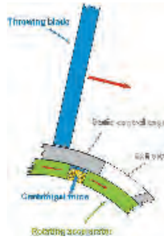
Fig.6 Elements involved in shot cohort transfer to throwing blade.
