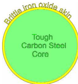
Fig.1 Section of spherical carbon steel shot particle.
