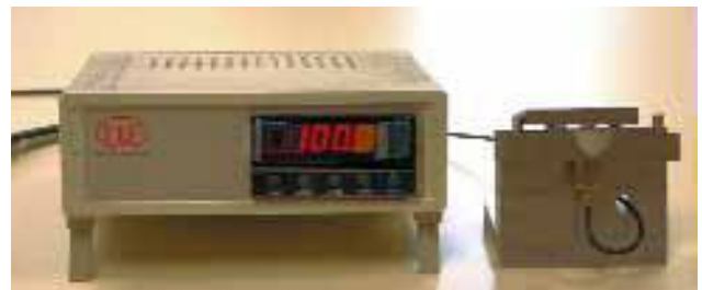
Figure 3. An EI "super" gage with .01000 " certified step block. EI has two super gages that measure prebowl to a resolution of 0.00001 " and meet SAE J 442 and AMS 2430 for #2 Almen gages. The readings from the gages are continually compared and monitored for accuracy.
