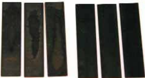
Figure 2. When strips were pulled from the box, it was even more obvious that they were from different manufacturing processes. Note the oil stains on the strips on the left.
