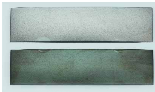
Figure 1. These strips underwent the same peening process. Verification of uniform coverage is easier on the new strip with Coverage Check Finish than on the darker, mottled strip.
