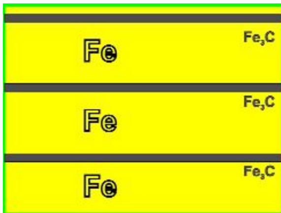
Fig.4 Schematic representation of “Pearlite” structure.
