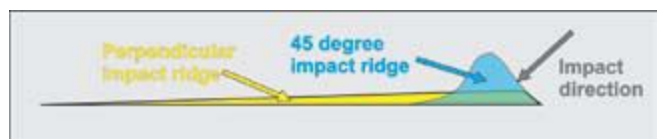
Fig.6. Comparison of perpendicular and 45o dent ridges.
