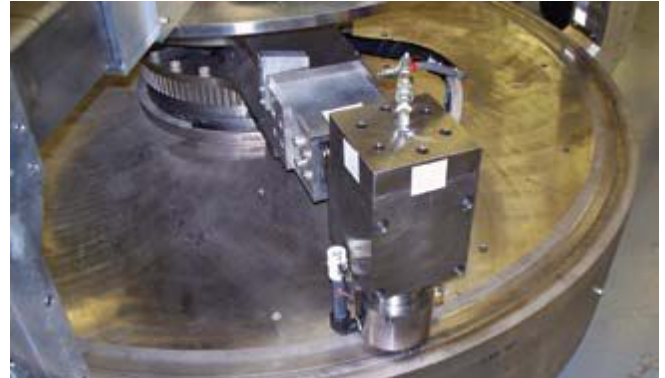
Figure 3: LPB Processing of Nuclear Waste Container Weld
