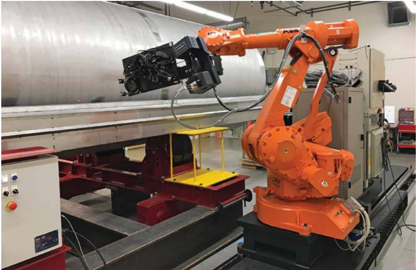
The laser peening process in development and testing with a Holtec Multi-Purpose Canister at the CWST facility in Livermore, California.
