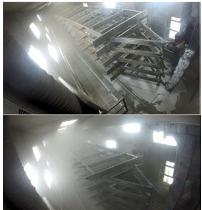
AMAGRIT is cleaner due to its low breakdown rate. AMAGRIT was used in the top blasting operation and AlOx in the bottom operation.
