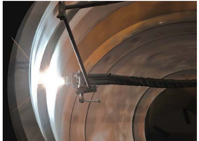
Arc Spraying on ID of Large Housing
