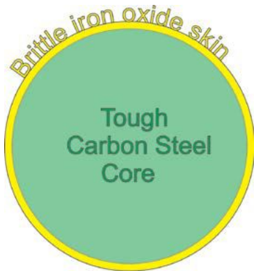
Fig.6. Iron oxide skin on carbon steel core.
