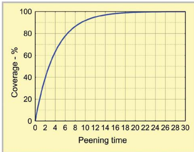
Fig.4. Effect of peening time on average coverage.
