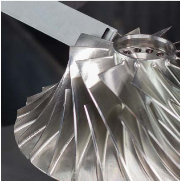
Figure 3: Efficient peening with specified nozzles and peening media
