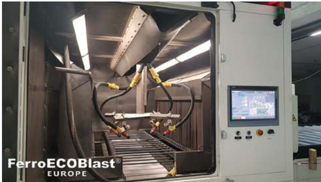
Manipulator with adjustable nozzles inside the machine
