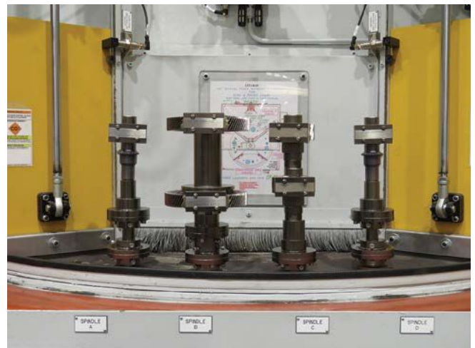
The 72" Flex Peener™ can shotpeen different-sized gears at the same time. (Shown here with Almen strip fixtures.)
