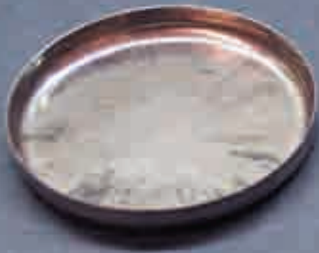
On the left is a net-shape form produced by LMC, Inc. from titanium powder from International Titanium Powder LLC. Read more about these companies and their new titanium technology center on page 4.
