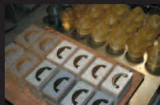
Urethane casting production
