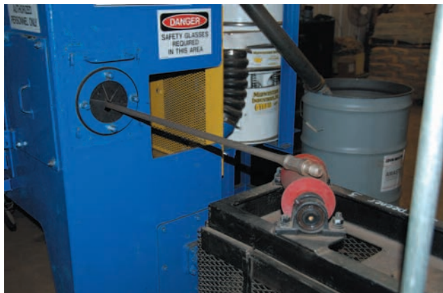
A sucker rod is fed into the Wheelabrator shot peen machine
