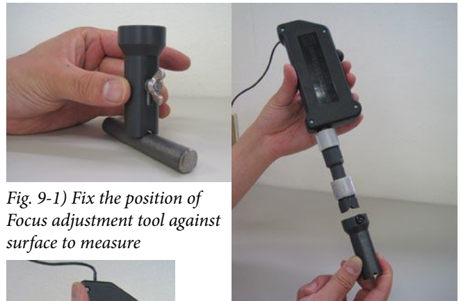
Fig. 9-2) Adjust the nozzle length with Focus adjustment tool
