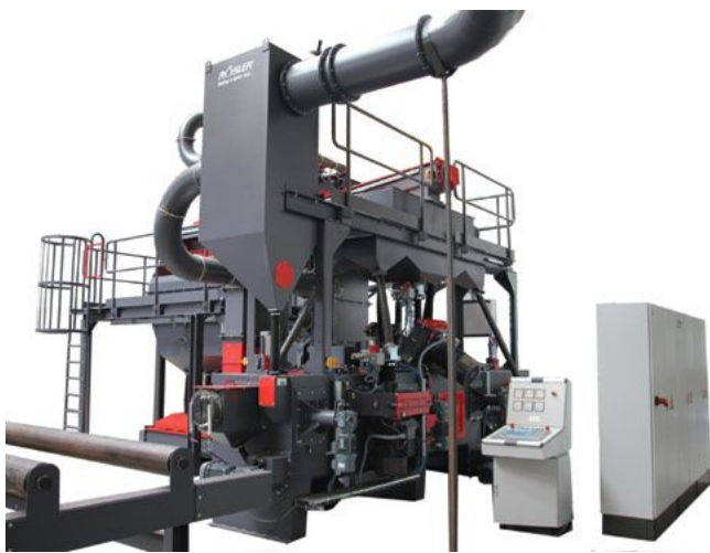
In this continuous shot blast machine with three blast chambers, steel bars with round, square and hexagonal profiles and diameters/cross-sectional dimensions from 24 to 80 mm (1.0 to 3.2 inches) can be processed at a speed from 12 to 60 m (39 to 197 feet) per minute.
