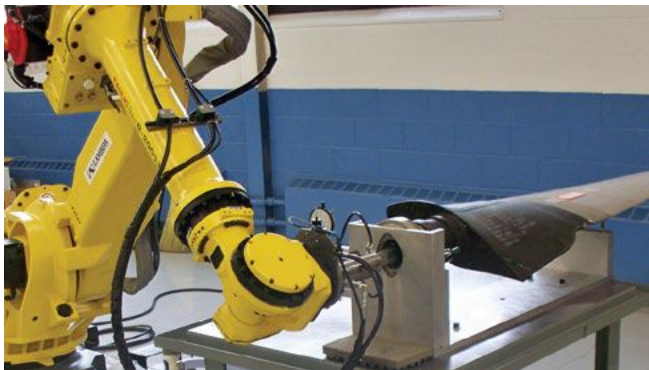
Robotic Processing of the P-3 Propeller Bore
