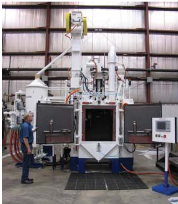
Single Cell Unit, 5 Pressure Nozzles
