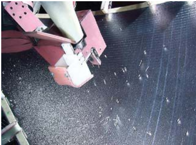
Peen forming of a tank bulkhead segment for Ariane 5.
