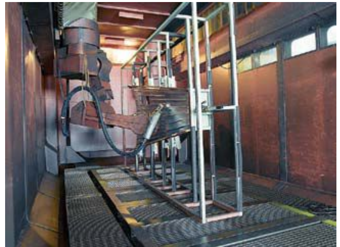
KSA's peen forming processes are fully automated.
