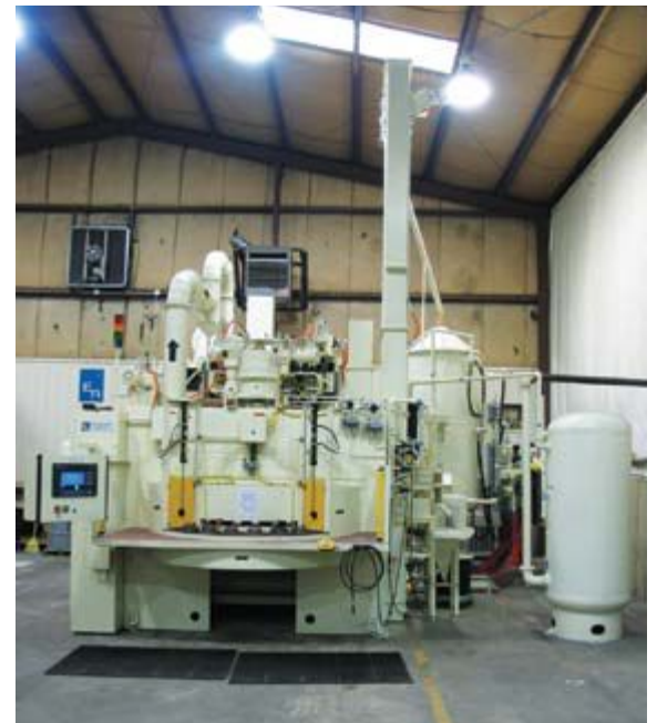
Large 84" Index Unit, 12 Pressure Nozzles
