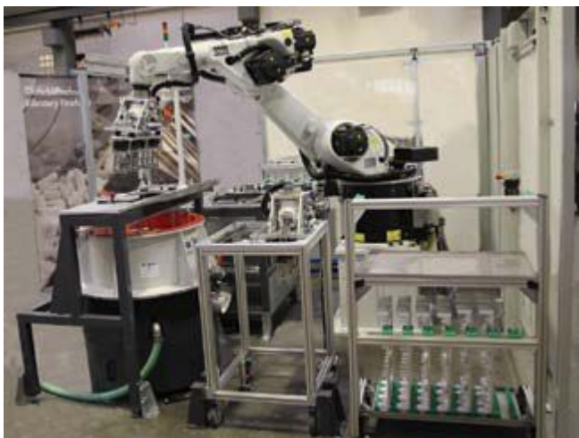
High-Frequency-Finishing (HFF), a newly developed vibratory finishing process produces excellent and absolutely repeatable deburring and polishing results in very short cycle times.
