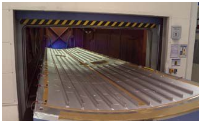
Automated peen re-shaping of a fuselage shell.
