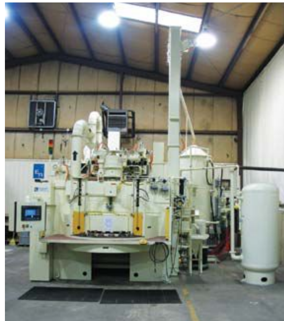
Large 84" Index Unit, 12 Pressure Nozzles
