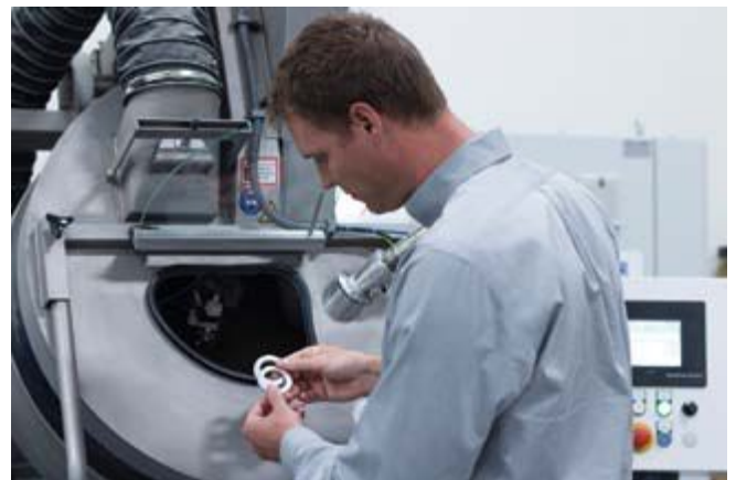
The Test & Training Centre in Grand Rapids is equipped with a Rotamat coater for coating of mass produced small parts.
