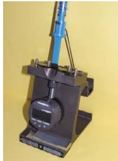
Fig.14. Force meter gauging response of an Almen strip.
