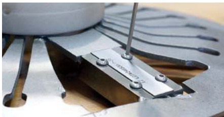
Part verification tool with Almen strip holder
