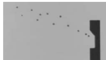
Flight direction and speed analysis at a blast lance for internal peening
