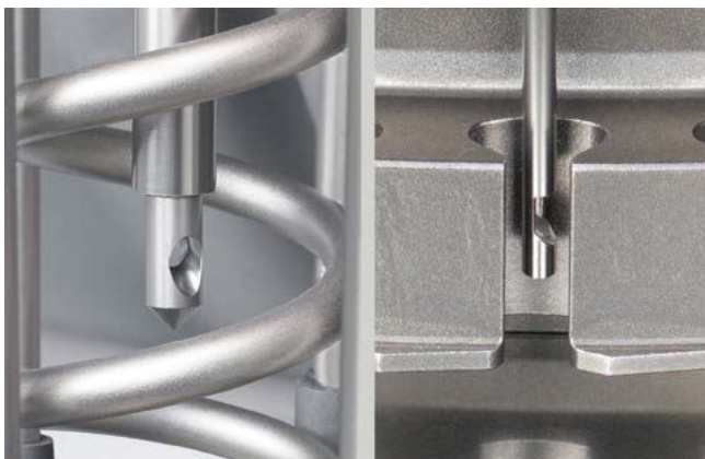
Internal peening of a coil spring | Internal peening of blade slots in a rotor
