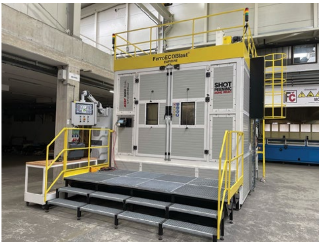
ARSP 1000 DUAL shot peening machine
