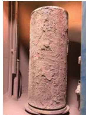
"Before" and "After" photographs of a cartridge-type filter. It has been cleaned with air, inspected, tested, and is ready for shipment back to the client.
