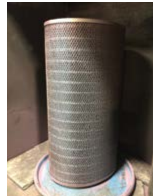
"Before" and "After" photographs of a cartridge-type filter. It has been cleaned with air, inspected, tested, and is ready for shipment back to the client.
