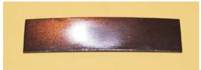
Fig.9. Hand-polished Almen ‘A’ strip showing area of complete indentation removal.
