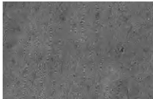
Figure 2. (After) This SEM photomicrograph (500X magnification) was taken after processing the same turbine blade in a multi-step procedure utilizing centrifugal barrel methods with both grinding and polishing free abrasive materials in sequence. The surface profile has been reduced from the original 75 - 90 Ra ( \mu\text{in} ) to a 5-9 Ra ( \mu\text{in} ) range. Additionally, there has been a plateauing of the surface and the resultant smoother surface manifests a negative skew ( R_s k ) instead of a positive skew. This type of surface is considered to be very "functional" in both the fluid and aerodynamic sense. The smooth, less turbulent flow created by this type of surface is preferred in many aerodynamic, automotive and other high force loading applications. Another important consideration the photomicrographs indicate is that surface and sub-surface fractures seem to have been removed. Observations with backscatter emission with a scanning electron microscope (SEM) gave no indication of residual fractures.
