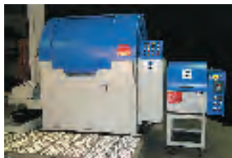
Figure 5. Centrifugal barrel machines such as these can produce exceptional edge and surface finishes in very short cycle times. Accelerated process effects can be developed because of the high speed interaction between abrasive media and part surfaces, and because media interaction with parts are characterized by high pressure by virtue of the high
