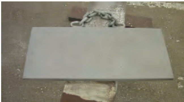
As part of the quality control process, the PMB operators blast a two-foot-wide aluminum coupon that has been covered with a paint similar to the coating on the shuttle.
