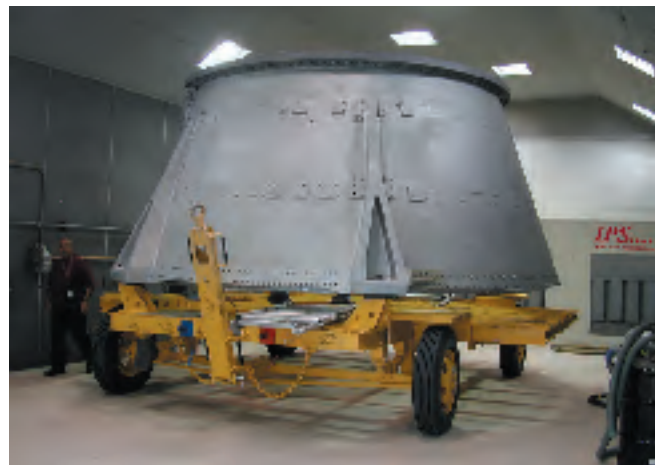
The shuttle's rocket booster nozzle inside the Innovative Peening Systems' PMB enclosure.
