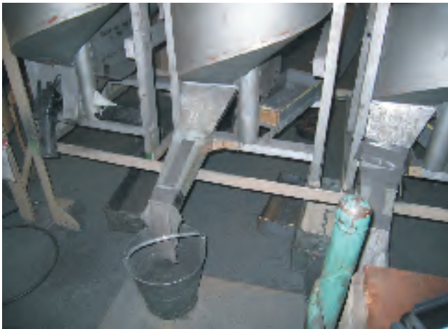
Fig.12 Segregation of acceptable and rejected shot fractions.
