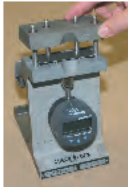
The Aero-Almen gage and aluminum strips provide a definitive measurement and quality control for the PMB process of the shuttles' solid rocket boosters.
