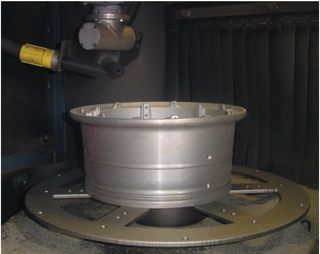
Part touched-up by nozzles after wheelblast
