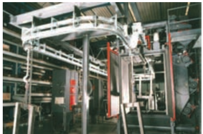
Because of the height adjustment of the monorail transport system, this continuous overhead monorail blast system can be easily loaded, either manually or by robot.
