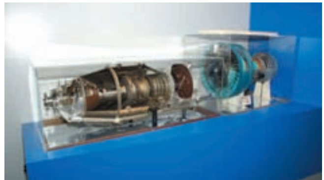
Left exhibit: Cut-out scaled model of Pratt & Whitney PT6A engine. Right exhibit: Scaled model of Pratt & Whitney PW4000 Turbofan engine.
