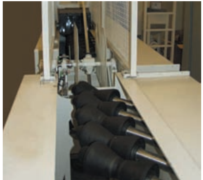
This skew roller conveyor moves the parts forward and rotates them at the same time.
