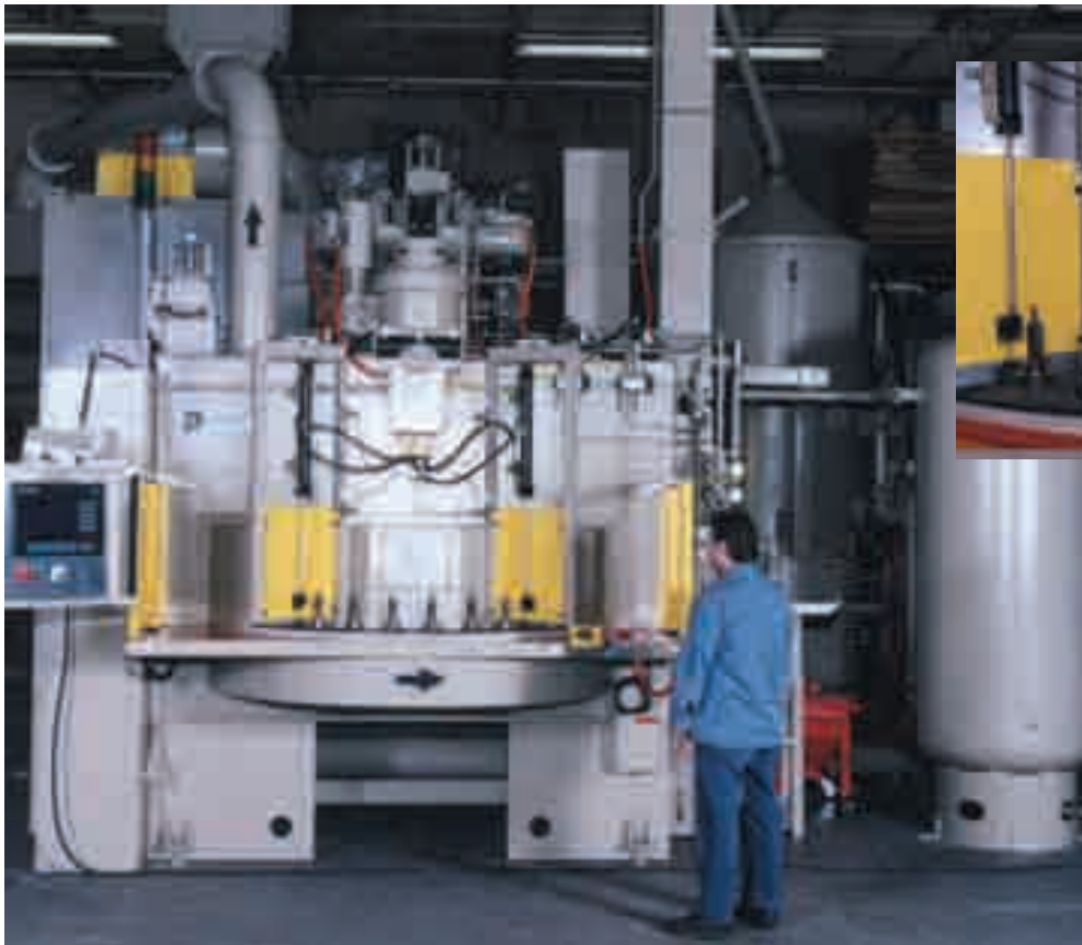
Patented 72" Index Unit with Shot Flow Controls, Sweco, Bucket Elevator, 12 Nozzles and 16 Spindles. Designed for automotive high-volume.
