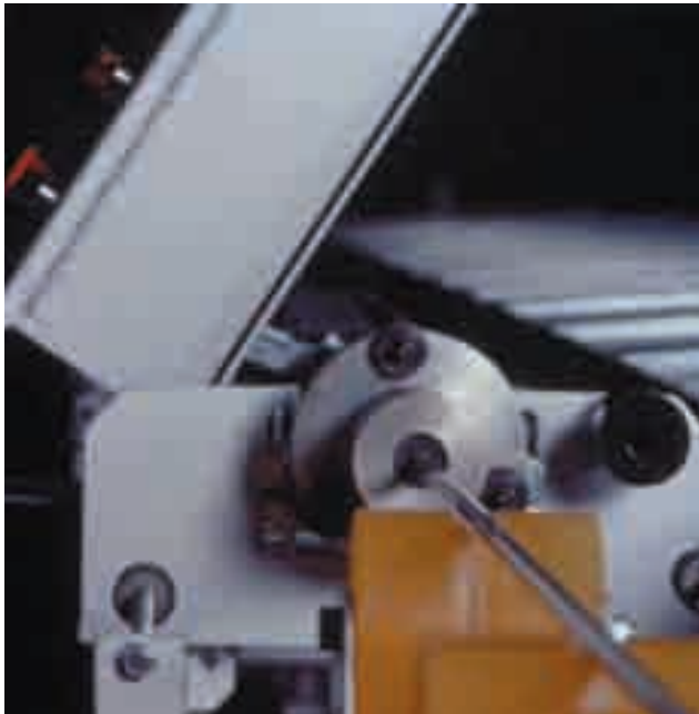
One of several special bolt-on nozzle adaptors, sized to suit tube ID, holds the tube in place at media-entry end.
