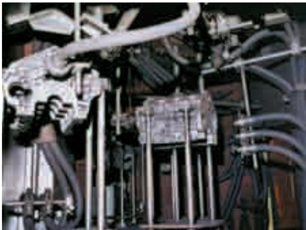
Each blasting station has 6 - 8 nozzles. Blasting is turned off at the end of each cycle so there is no wasted blast (i.e., no wasted media, excess energy usage or excess machine wear and tear).
