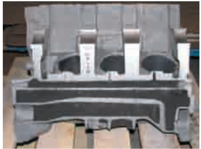
Before: A cross-section of an engine block casting before blast cleaning.
