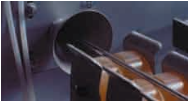
Tubes enter a sealed opening on the side of the cabinet ensuring that media and dust are contained in the enclosure.
