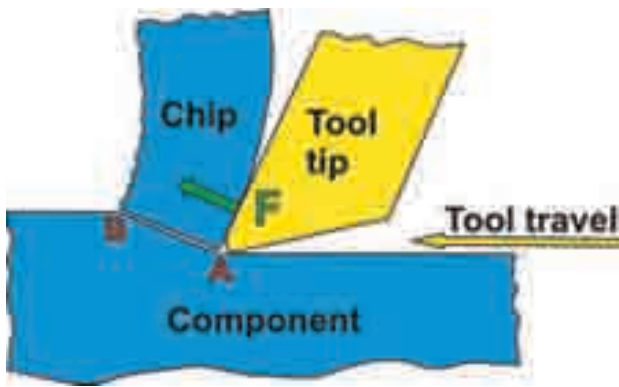
Fig.2 Chip formation during machining.
