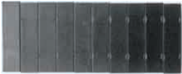
Fig.9 Scanned image of a set of pre-polished Almen strips having progressive peening levels.
