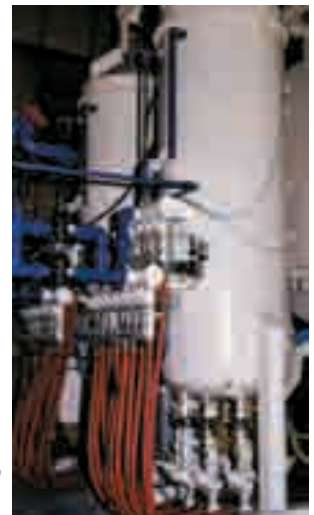
Each pressure vessel holds up to 30,000 lbs of shot.
