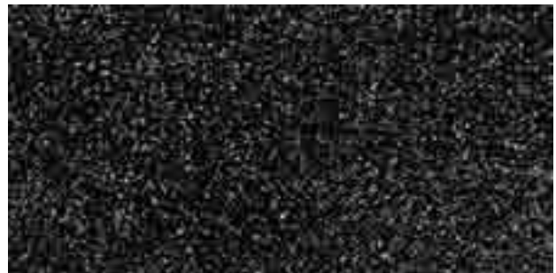
Fig.8 Scanned image of Almen strip peened with S230, x8, 1200 dpi.
