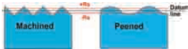
Fig.3 Comparison of machined and peened surface cross-sections.
