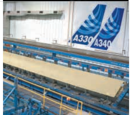
Photo: Airbus A330/A340 upper panels at Vought
