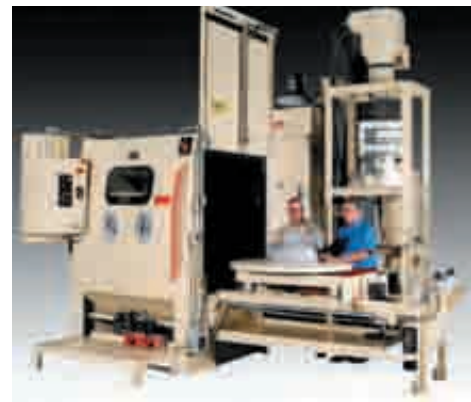
(Fig. 2) Robert Heaton, product support manager (right) and Dan Herbert, product manager, put a piece of custom equipment through its paces prior to shipping. Test blasting demonstrated the ability of this single system to process a long list of customer parts to spec and on budget.
