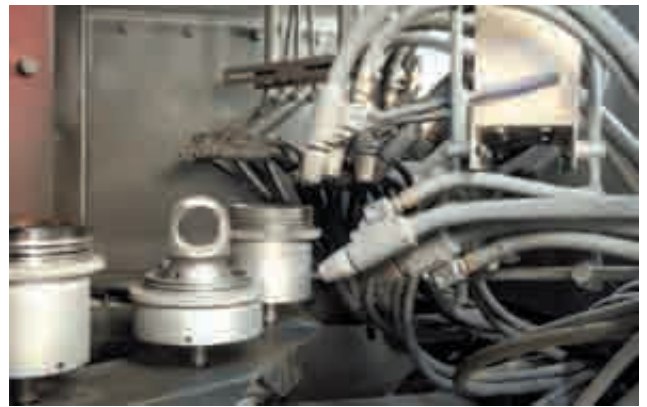
(Fig. 5) Blast system coordinates movements of 16 blast guns, oscillating vertically and horizontally, with spinning stations on a rotating platform. Eight guns oscillating vertically clean the sides and skirts of pistons. Guns sweeping horizontally clean tops and interiors.
