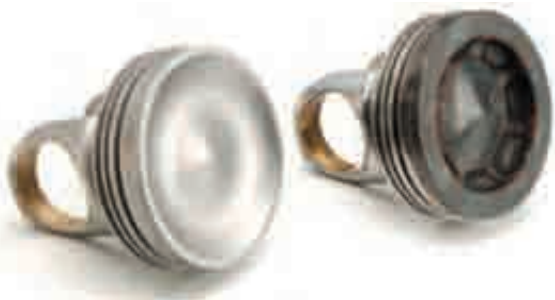
(Fig. 4) Lab work and number crunching found improved tactics for cleaning pistons. Less pressure and more expensive media reduced per-unit costs by 30%.
