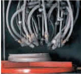
(Fig. 3) Rotary blast heads provide broad coverage while conserving compressed air. Available with up to nine guns, these rotating heads improve efficiency in many in-line, turntable and batch air-blast systems.
