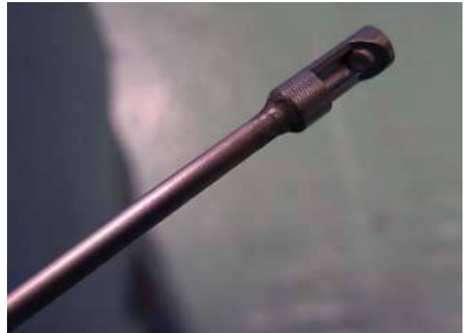
Fig.3 Nozzle for internal surface
