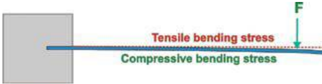
Fig.5. Shot stream applying a force, F , to an end-clamped strip.
