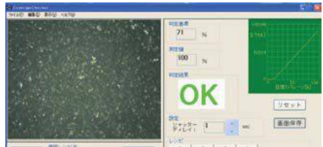
Fig.2 Quantifying blasted area by Coverage Checker™
