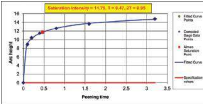
Fig.12. Analyzed Saturation curve for A strips using same peening conditions as for fig.10.
