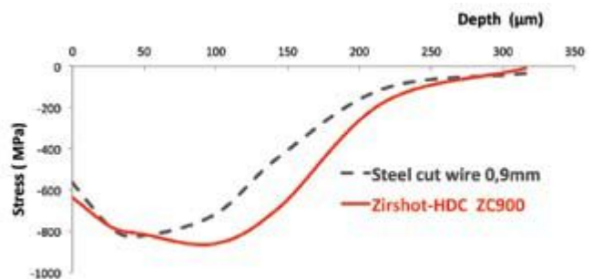
Figure 2. Steel surface peened with Zirshot® HDC
