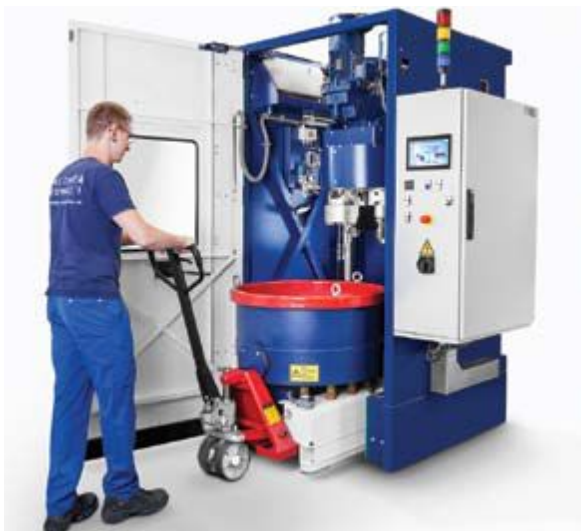
Work bowls containing different media types can be easily and quickly exchanged with a pallet truck.
