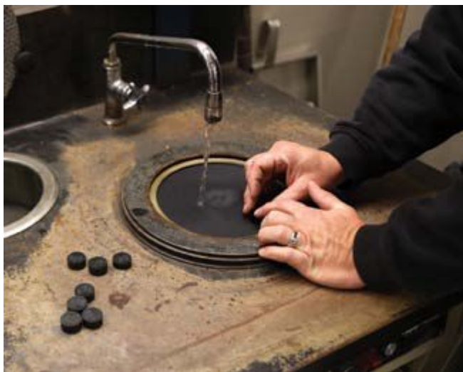
Hardness Testing – Shot grains are captured in a Bakelite Base and ground to half their diameter. Hardness is tested at the center.
