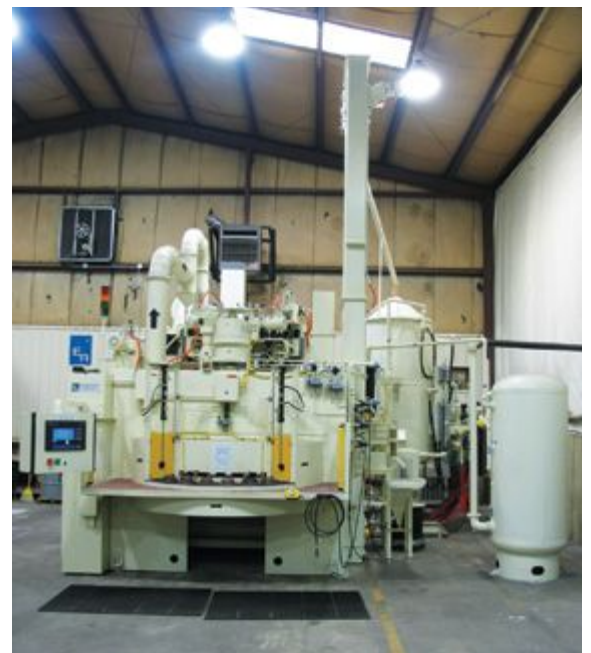
Large 84" Index Unit, 12 Pressure Nozzles
