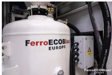
Double-chamber pressure peening generator of ARSP 1000 ECO DUAL
