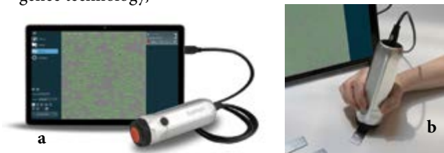
Fig. 1 (a) The GelSight Mobile™ system.
